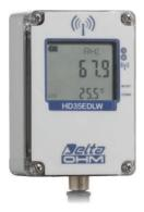
Temperature and humidity wireless data logger. **IP 67** waterproof housing. Custom LCD display (only with **option L**). It stores the measures in its internal memory (24,000 samples) and transmits the logged data to the base unit automatically at regular intervals or upon request.
