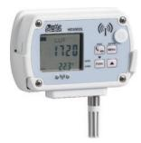
Temperature, humidity, atmospheric pressure, illuminance and UVA irradiance wireless data logger. Custom LCD display (only with **option L**). It stores the measures in its internal memory (32,000 samples) and transmits the logged data to the base unit automatically at regular intervals or upon request.
