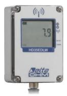
Rainfall quantity wireless data logger. **IP 67** waterproof housing. Custom LCD display (only with **option L**). It stores the measures in its internal memory (36,000 samples) and transmits the logged data to the base unit automatically at regular intervals or upon request.
