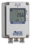
Temperature wireless data logger. **IP 67** waterproof housing. Custom LCD display (only with **option L**). It stores the measures in its internal memory (from 42,000 to 68,000 samples depending on the number of inputs) and transmits the logged data to the base unit automatically at regular intervals or upon request.
