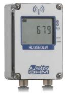
Solar radiation and rainfall quantity wireless data logger. IP 67 waterproof housing. Custom LCD display (only with option L). It stores the measures in its internal memory and transmits the logged data to the base unit automatically at regular intervals or upon request.
