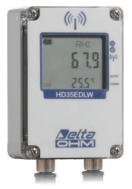
Temperature and humidity and leaf wetness wireless data logger. **IP 67** waterproof housing. Custom LCD display (only with **option L**). It stores the measures in its internal memory (22,000 samples) and transmits the logged data to the base unit automatically at regular intervals or upon request.
