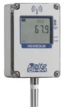
Humidity wireless data logger. **IP 67** waterproof housing. Custom LCD display (only with **option L**). It stores the measures in its internal memory (68,000 samples) and transmits the logged data to the base unit automatically at regular intervals or upon request.
