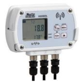
Temperature wireless data logger. Custom LCD display (only with **option L**). It stores the measures in its internal memory (from 42,000 to 68,000 samples depending on the number of inputs) and transmits the logged data to the base unit automatically at regular intervals or upon request.
