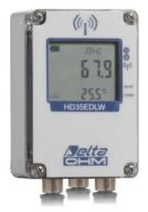
Environmental temperature, humidity, solar radiation and solar panel temperature wireless data logger. IP 67 waterproof housing. Custom LCD display (only with option L). It stores the measures in its internal memory (22,000 samples) and transmits the logged data to the base unit automatically at regular intervals or upon request.
