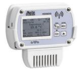
Temperature, humidity, carbon monoxide and dioxide wireless data logger. Graphic LCD display (only with **option G**). It stores the measures in its internal memory (36,000 samples) and transmits the logged data to the base unit automatically at regular intervals or upon request.
