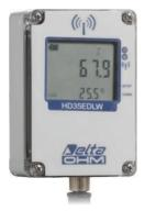
Soil temperature and humidity wireless data logger. **IP 67** waterproof housing. Custom LCD display (only with **option L**). It stores the measures in its internal memory (52,000 samples) and transmits the logged data to the base unit automatically at regular intervals or upon request.
