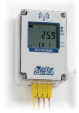
Temperature wireless data logger. **IP 67** waterproof housing. Custom LCD display (only with **option L**). It stores the measures in its internal memory (from 36.000 to 68.000 samples depending on the number of inputs used) and transmits the logged data to the base unit automatically at regular intervals or upon request.
