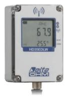
Temperature, humidity and atmospheric pressure wireless data logger. **IP 67** waterproof housing. Custom LCD display (only with **option L**). It stores the measures in its internal memory (22,000 samples) and transmits the logged data to the base unit automatically at regular intervals or upon request.
