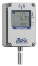
Temperature and humidity wireless data logger. **IP 67** waterproof housing. Custom LCD display (only with **option L**). It stores the measures in its internal memory (24,000 samples) and transmits the logged data to the base unit automatically at regular intervals or upon request.
