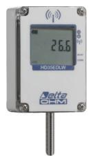
Temperature wireless data logger for freezing tunnels. **IP 67** waterproof housing. Custom LCD display (only with **option L**). It stores the measures in its internal memory (68,000 samples) and transmits the logged data to the base unit automatically at regular intervals or upon request.
