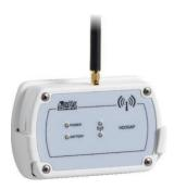
Device acting as an interface between the network data loggers that are positioned in the measurement sites, and the PC/PLC. It receives via wireless the data acquired by the remote data loggers and communicate with the PC/PLC via the **USB** output or the **Ethernet** or **Wi-Fi** local network.
