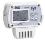
Temperature, humidity, atmospheric pressure, carbon monoxide and dioxide wireless data logger. Graphic LCD display (only with **option G**). It stores the measures in its internal memory (32,000 samples) and transmits the logged data to the base unit automatically at regular intervals or upon request.
