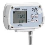
Temperature, humidity, atmospheric pressure and illuminance wireless data logger. Custom LCD display (only with **option L**). It stores the measures in its internal memory (36,000 samples) and transmits the logged data to the base unit automatically at regular intervals or upon request.
