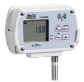
Temperature wireless data logger. Custom LCD display (only with **option L**). It stores the measures in its internal memory (68,000 samples) and transmits the logged data to the base unit automatically at regular intervals or upon request.
