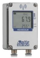
Temperature and humidity wireless data logger. **IP 67** waterproof housing. Custom LCD display (only with **option L**). It stores the measures in its internal memory (22,000 samples) and transmits the logged data to the base unit automatically at regular intervals or upon request.
