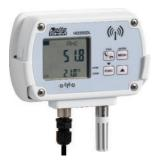
Temperature, humidity, atmospheric pressure, illuminance and UVA irradiance wireless data logger. Custom LCD display (only with **option L**). It stores the measures in its internal memory (32,000 samples) and transmits the logged data to the base unit automatically at regular intervals or upon request.
