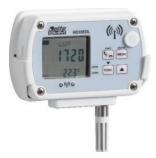
Temperature, humidity and illuminance wireless data logger. Custom LCD display (only with **option L**). It stores the measures in its internal memory (44,000 samples) and transmits the logged data to the base unit automatically at regular intervals or upon request.
