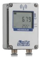
Solar radiation and solar panel temperature wireless data logger. **IP 67** waterproof housing. Custom LCD display (only with **option L**). It stores the measures in its internal memory (36,000 samples) and transmits the logged data to the base unit automatically at regular intervals or upon request.
