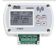
Wireless data logger with three terminal header inputs for the connection of transmitters with  $4\div20\,$  mA,  $0\div1\,$  V or  $0\div50\,$  mV output, Pt100/Pt1000 sensors, K, J, T, N, E thermocouples, sensors with voltage free contact output (max. one sensor) and potentiometric sensors.
