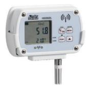
Temperature and humidity wireless data logger. Custom LCD display (only with **option L**). It stores the measures in its internal memory (24,000 samples) and transmits the logged data to the base unit automatically at regular intervals or upon request.
