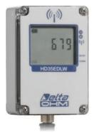
Solar radiation wireless data logger. **IP 67** waterproof housing. Custom LCD display (only with **option L**). It stores the measures in its internal memory (42,000 samples) and transmits the logged data to the base unit automatically at regular intervals or upon request.
