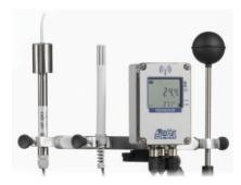
Wireless data logger for the analysis of the **WBGT** (Wet Bulb Globe Temperature) index. **IP 67** waterproof housing. Custom LCD display (only with **option L**). It stores the measures in its internal memory (30,000 samples) and transmits the logged data to the base unit automatically at regular intervals or upon request.
