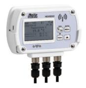
Temperature wireless data logger. Graphic LCD display (only with **option G**). It stores the measures in its internal memory (from 42,000 to 68,000 samples depending on the number of inputs) and transmits the logged data to the base unit automatically at regular intervals or upon request.
