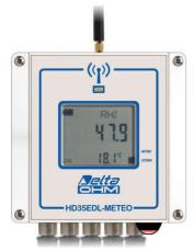
Temperature, humidity, atmospheric pressure, solar radiation, rainfall quantity, wind speed and direction wireless data logger. **IP 67** waterproof housing. Custom LCD display (only with **option L**). It stores the measures in its internal memory (from 28,000 to 58,000 samples depending on the number of inputs used) and transmits the logged data to the base unit automatically at regular intervals or upon request.
