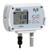
Temperature, humidity, illuminance and UVA irradiance wireless data logger. Custom LCD display (only with **option L**). It stores the measures in its internal memory (32,000 samples) and transmits the logged data to the base unit automatically at regular intervals or upon request.
